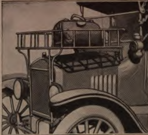
A Metal Rack, Placed over the Hood as a Baggage Carrier, Is Both a Convenience and an Advertisement for the Proprietor of the Hotel
